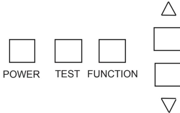
**POWER:** Press and hold for 3 seconds to turn the unit ON. Once on, press and hold the button for two seconds to turn the backlight ON. Press and hold the button for 4 seconds to turn the unit OFF.
